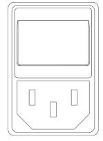
Turn the power switch to the "on" position and the unit's air compressor will cycle on.
