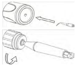
\*To remove sclaer handpiece from tubing, Gently pull straight off. Don't turn / twist or damage to tubing pins will occur.
